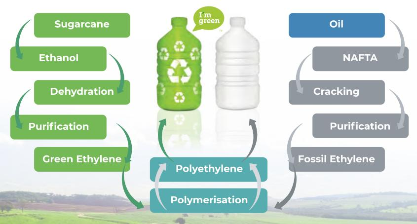
Technology: The production route for green polyethylene and the fossil polyethylene are the same, therefore the green polymer has got the same characteristics, quality and properties as the fossil equivalent.
